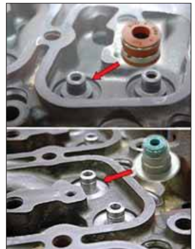
Figure 9 The upper image shows the early design seal with sharp machining edges in spring pocket area. The lower images show top hat type seal with radius spring pocket area.
