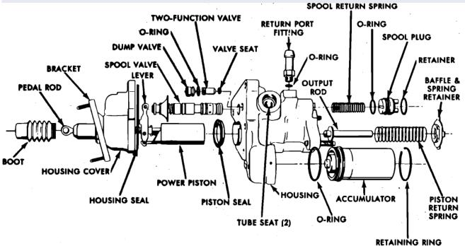
The Hydro-Boost system, provides an additional cylinder in the brake system. This cylinder contains no brake fluid. The Hydro-Boost cylinder is hydraulically
