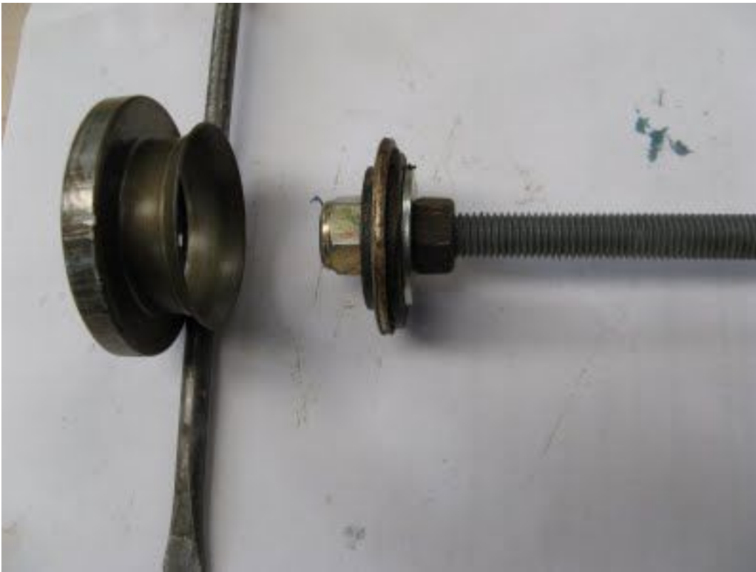
The pusher for removing the inner seals and cleaning out the axle tubes.
