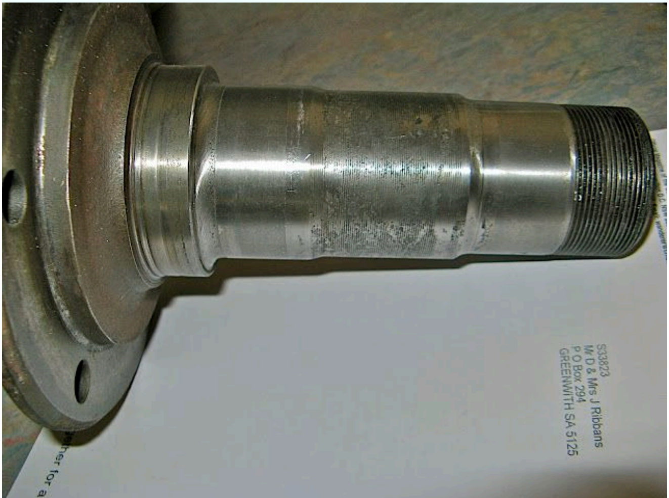
Pic 2. The repaired spindle. Bearings are a good tight slide fit on the reground shafts.
