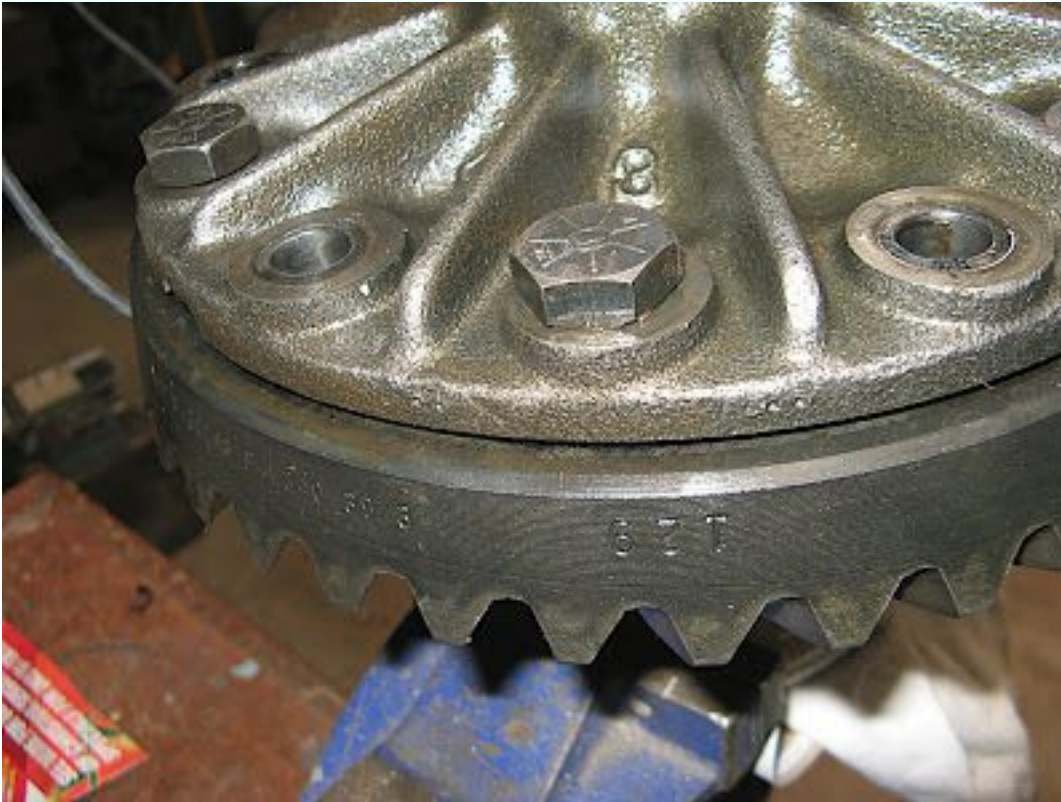
The Ring Gear being removed.
