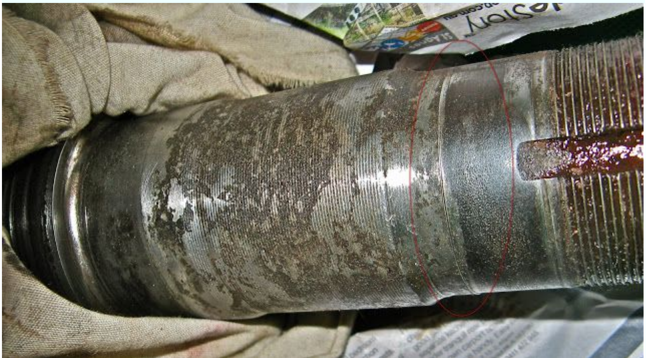
Pic 1. The groove and ridge ringed on the spindle shaft. (Click to enlarge)
