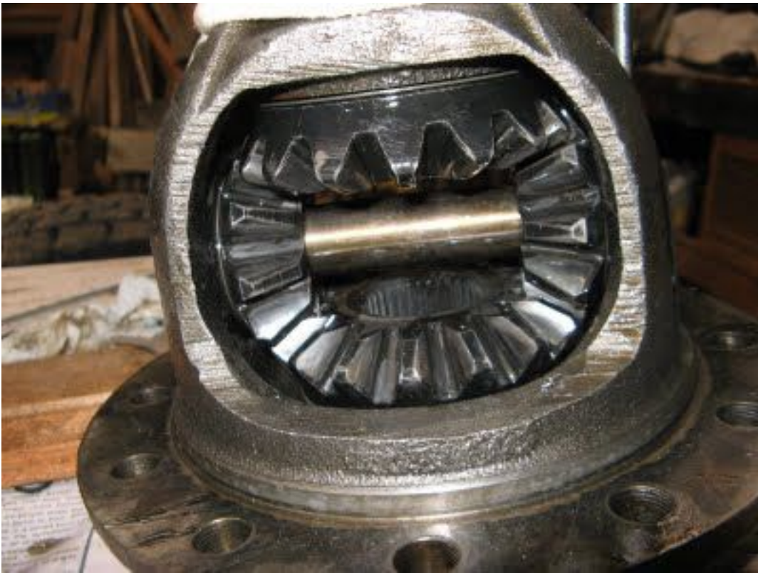
Gears reinstalled in the carrier.
