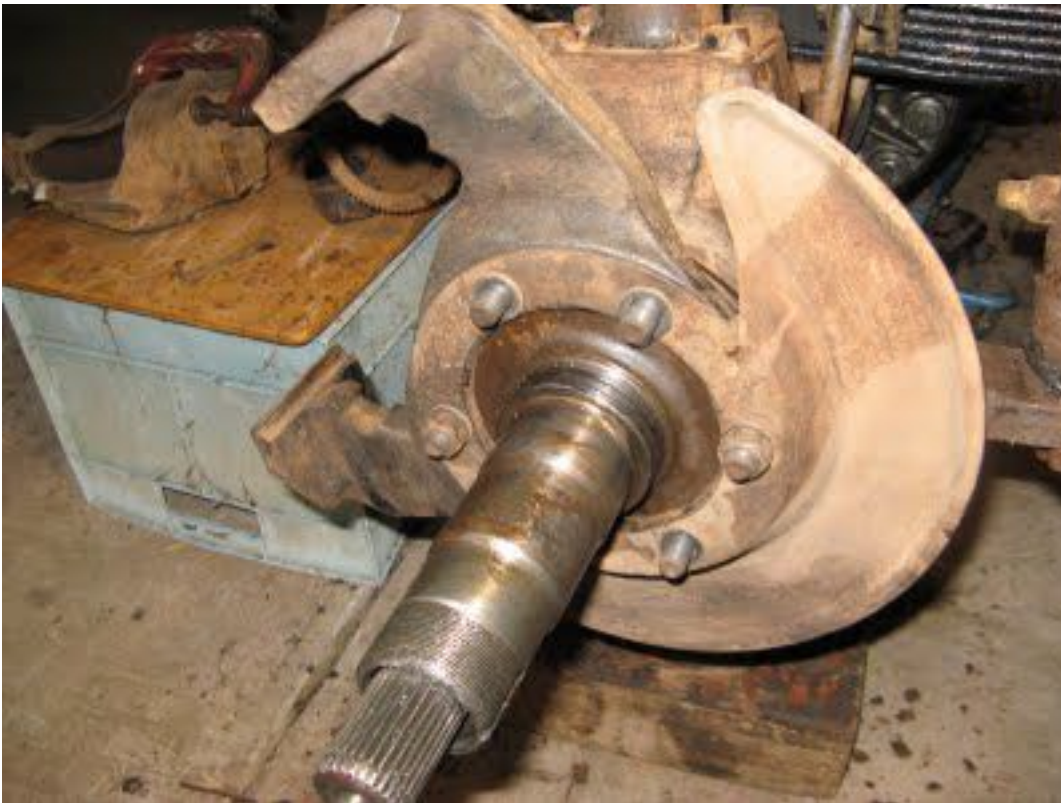
Refitting the Spindle, drivers side.
