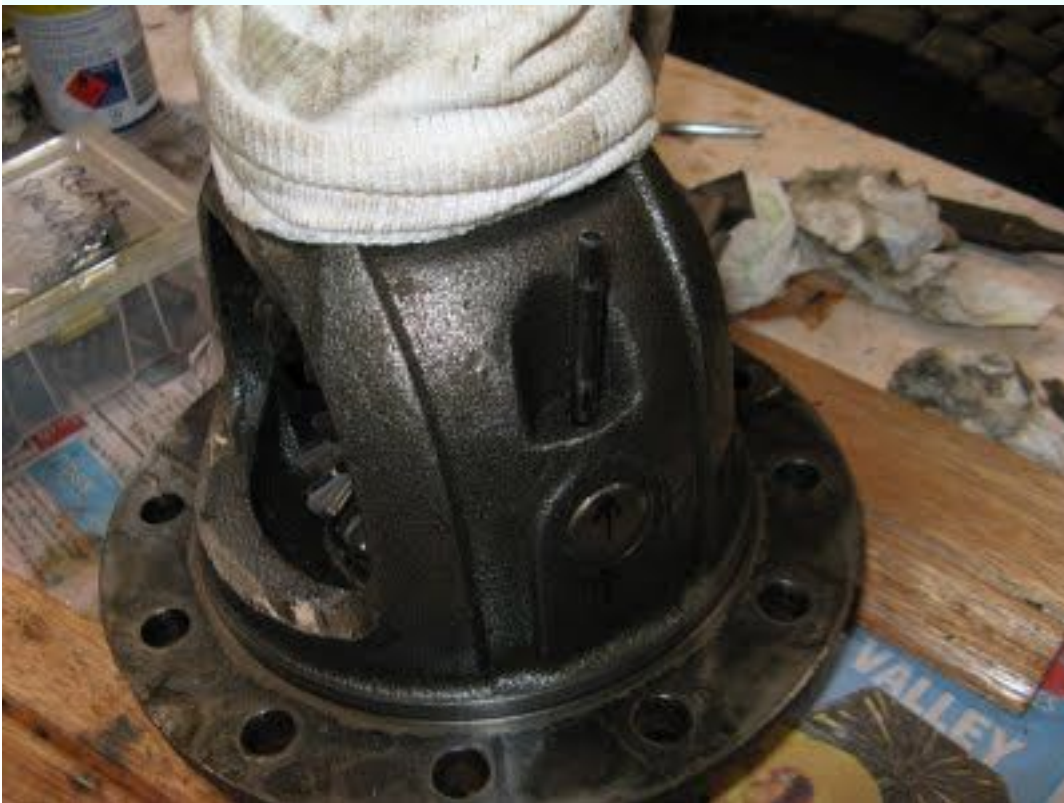
Driving the Roll Pin home to complete the assembly.
