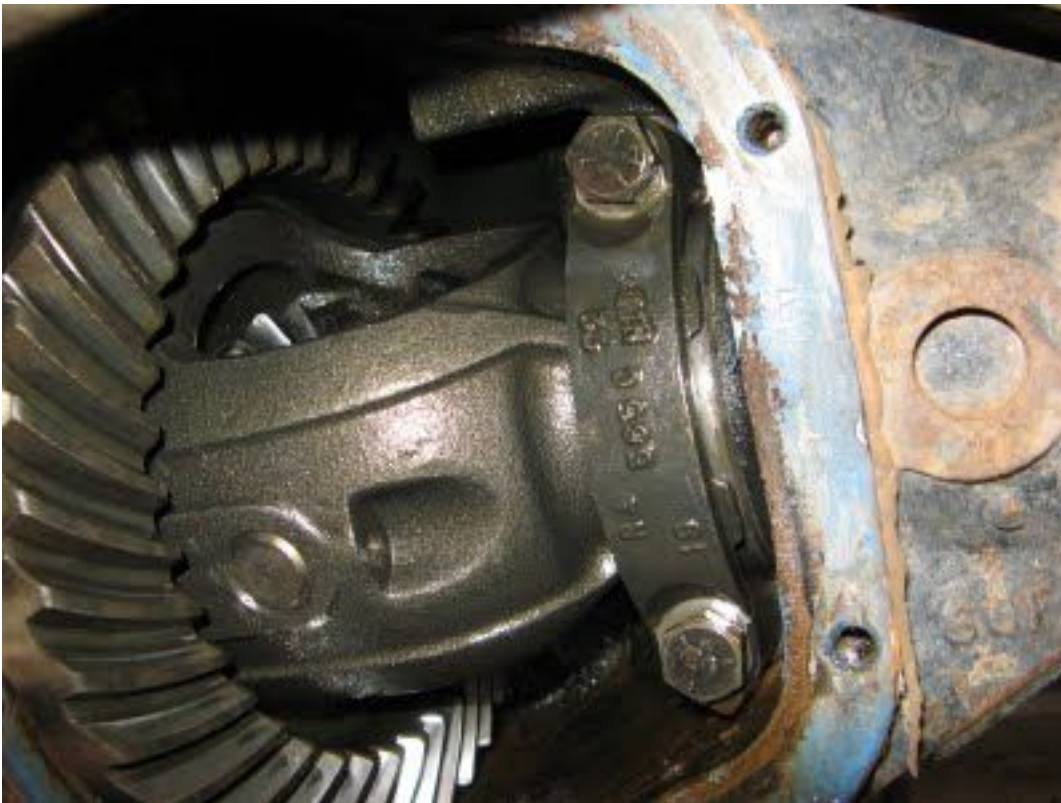
The differential installed in the carrier.
