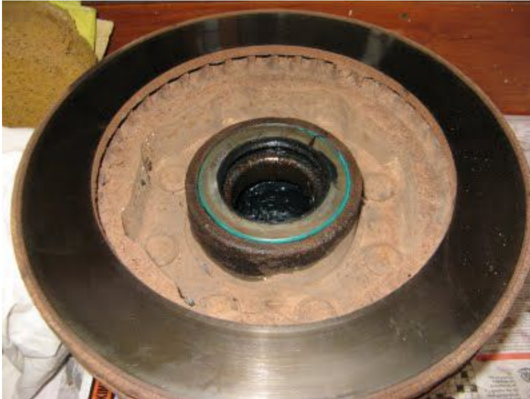
Oil seal inserted into the rear of the hub.
